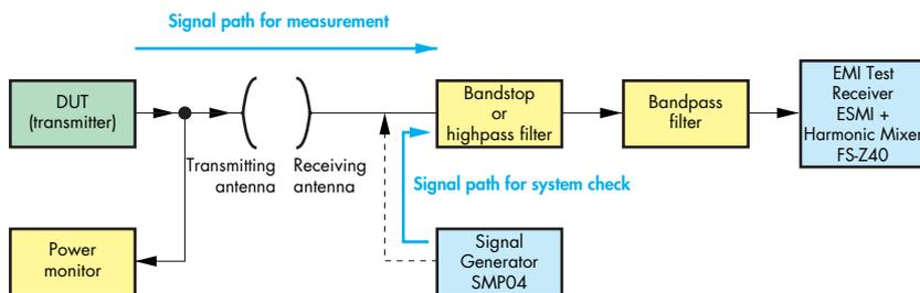
Normally, frequency drifts in RF cables, power amplifiers and the antenna of the test setup cause considerable level errors. This cannot be avoided in spite of the excellent level accuracy of SMP (typical error 0.1 dB). Fortunately, SMP does have a number of **functions for frequency response correction**:
