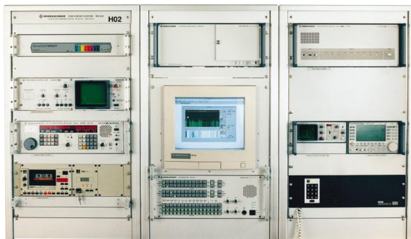
FIG 1 Radiomonitoring System RAMON-search with application-specific add-ons as desktop Photo 42 134/2
