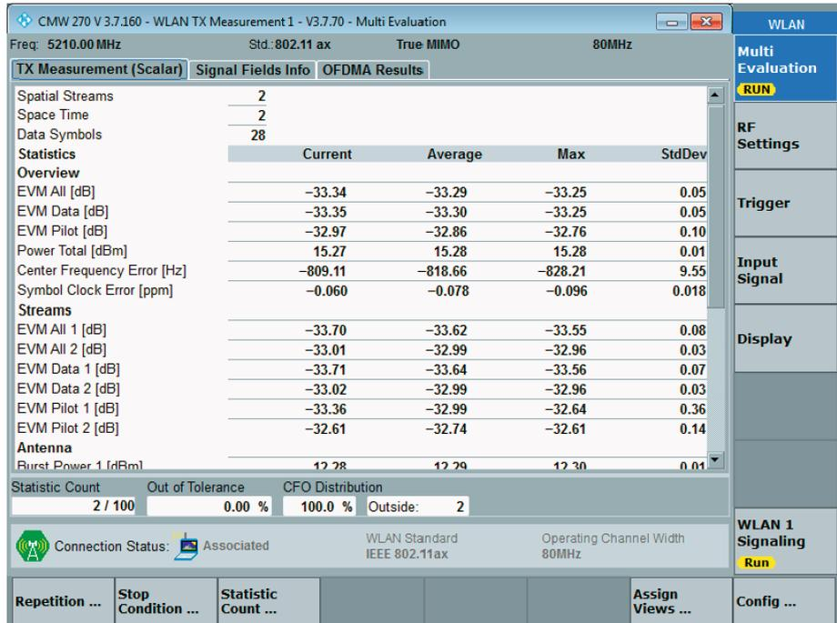
Fig. 5: The error vector measurement (EVM) makes it possible to evaluate a transmitter’s modulation accuracy. Here, the measurement is performed simultaneously for both MIMO transmitter paths. Depending on the modulation and coding, different limits are defined in the standard.
