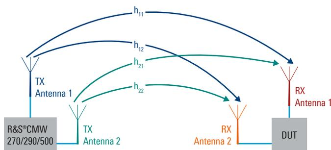
Fig. 1: In spatial multiplexing, each receive antenna receives a sum signal consisting of all of the transmitted signals. The prevailing channel conditions are represented in a transmission matrix  $H$  with elements  $h_{nm}$ .
