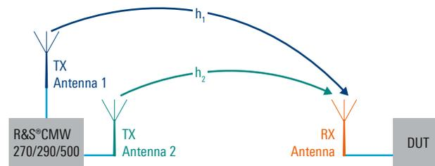
Fig. 2: In space time block coding, the modified outgoing data stream is transmitted via multiple antennas and received via a single antenna.
