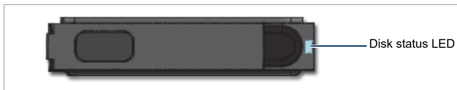
HB and EB drive carrier LEDs
