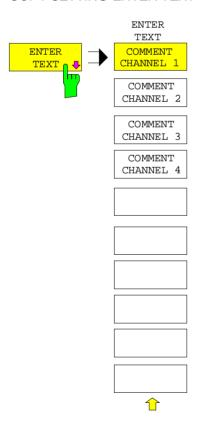
With the functions of the *ENTER TEXT* menu, commentary for individual diagrams can be entered. The comment text appears in the print-out, but does not appear on the display screen.
