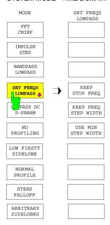
The SET FREQS LOWPASS softkey opens the submenu for determining the harmonic frequency grid required for the lowpass mode: A harmonic grid can be obtained in different ways:
