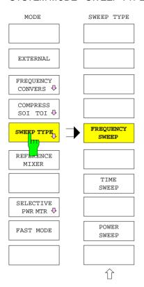
The SWEEP TYPE softkey opens the submenu for selecting the sweep variable. Possible sweep variables are sweeping frequency, time and power of the internal signal source. FREQUENCY SWEEP is the default setting.
