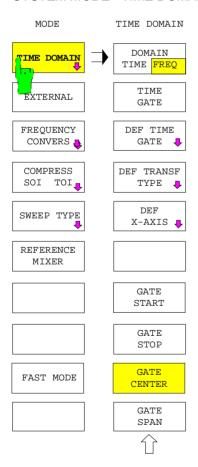
The *TIME DOMAIN* softkey opens the submenu for switching on/off and configuring the time-domain transformation mode. A prerequisite is that Time Domain option ZVR-B2 is installed.
