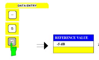
➤ Enter -5 via the numeric keypad and terminate the entry using the x1 key.
