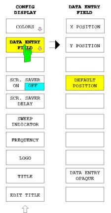
The DATA ENTRY FIELD softkey opens a submenu used to define the position of the selection tables and their display in opaque or transparent form.
