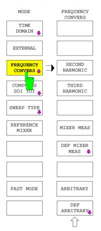
The FREQUENCY CONVERS softkey opens the submenu that activates, deactivates and configures frequency-converting measurements. The type of the frequency conversion is defined relative to a **base frequency**.
