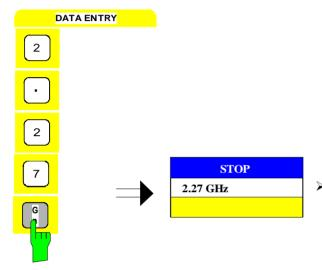
➤ Enter 2.27 via the numeric keypad and terminate the entry using the G/n key.
