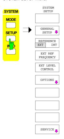
The SETUP key opens the menu for configuration of the instrument.
