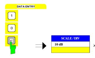
➤ Enter 10 via the numeric keypad and terminate the entry using the x1 key.
