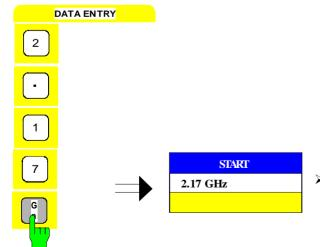
➤ Enter 2.17 via the numeric keypad and terminate the entry using the G/n key.
