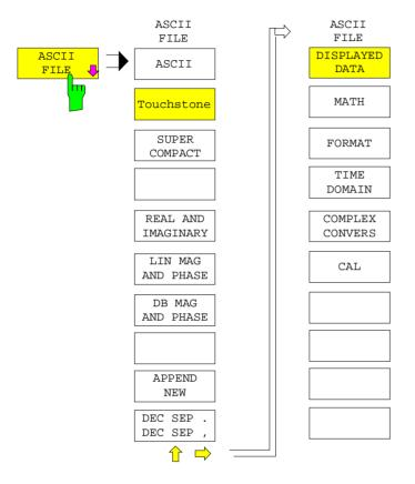
The ASCII FILES softkey opens a submenu used to define the characteristics of the ASCII file to be created.
