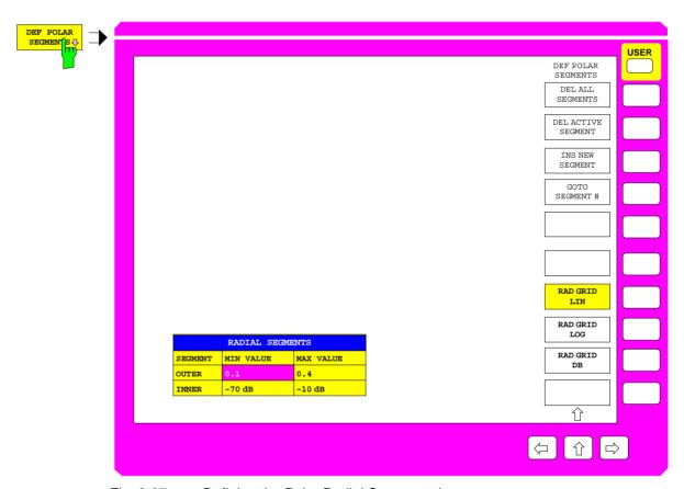
Fig. 2-37 Defining the Polar Radial Segmentation
