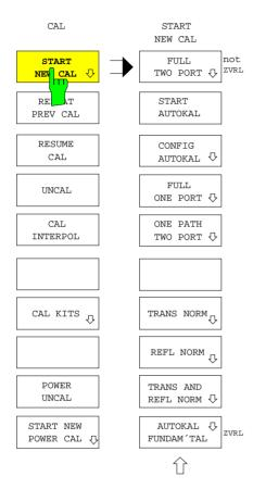
The START NEW CAL softkey starts the system-error calibration. The softkey calls a chain of submenus which leads back to the main menu of the CAL key after a completed calibration.
