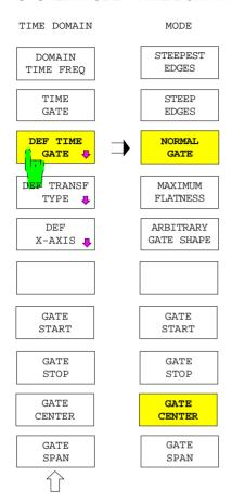
The *DEF TIME GATE* softkey opens the submenu for configuring the time domain gate:
