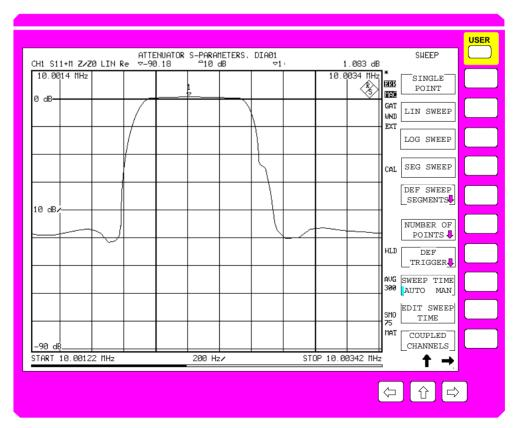
Fig. 2-14 Linear, Cartesian diagram
