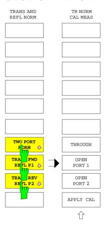
The TWO PORT NORM, TRANS FWD REFL P1 and TRANS REV REFL P2 softkeys open submenus for performing a combined as a bi-directional or unidirectional calibration in forward or reverse direction.
