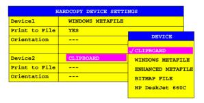
Three file formats and the Windows NT clipboard are always available, even if a printer has not yet been installed under Windows NT. All installed printers are listed below in alphabetic order.
