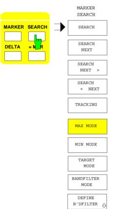
The functions of the MARKER SEARCH menu can be divided into functions which allow the search target to be defined and functions which actually trigger the defined search. Possible search targets are
