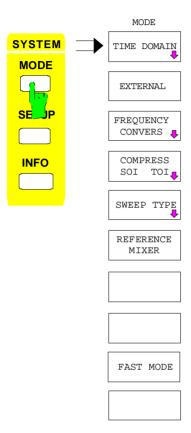
The *MODE* key opens the menu for setting the measuring mode of the network analyzer (NWA). Some of the modes require the installation of options.
