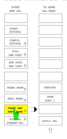
The TRANS AND REFL NORM softkey calls the menu for combined transmission and reflection normalization.
