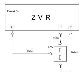
Block diagram for measuring the matching of input b1. For measurement of input b2, the connections from RVZ to Input b1/b2 are reversed.
