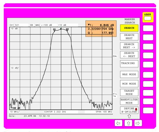
Fig. 2-9 Determination of the Q-factor
