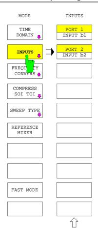
On a ZVK and ZVM, the INPUTS softkey appears in place of the EXTERNAL softkey provided at least one receiver attenuator is installed.
