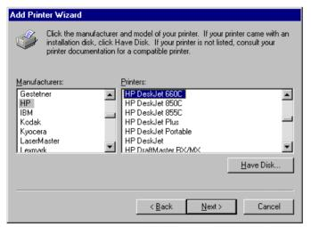
Mark the manufacturer in selection table "Manufacturers" and then the printer driver in selection table "Printers".
