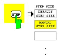
The STEP key opens the STEP menu for entry of the step size.
