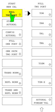
The *FULL TWO PORT* softkey selects the calibration mode complete two-port calibration.
