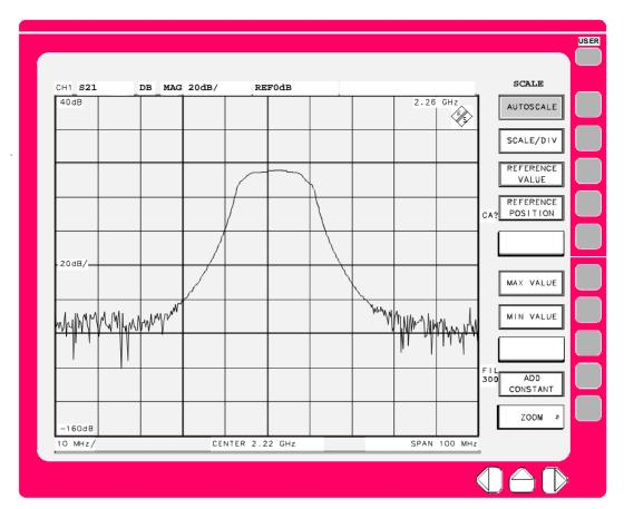
Fig. 2-1 Measurement display screen with an autoscaled trace
