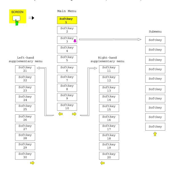
The menu arrows at the lower edge of the softkeys make it easier for the user to "navigate" through the menu tree.
