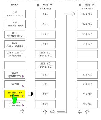
The Z AND Y PARAMS softkey opens a submenu for measuring two-port Z or Y parameters.
