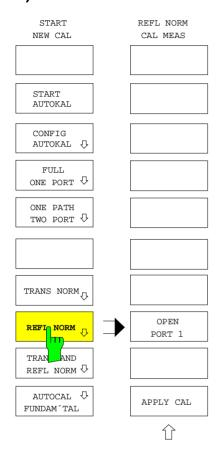
The *REFL NORM* softkey directly calls the menu for reflection normalization at test port 1.
