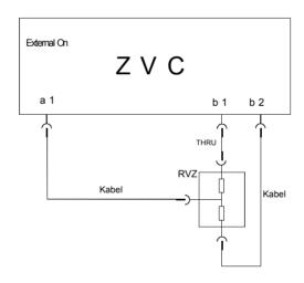
Block diagram for measuring the matching of input b1. For measurement of input b2, the connections from RVZ to Input b1/b2 are reversed.
