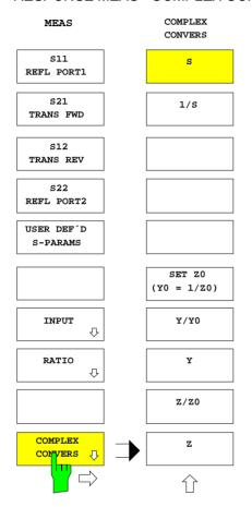
The *COMPLEX CONVERS* opens the submenu for selecting the conversion of the measured quantity.
