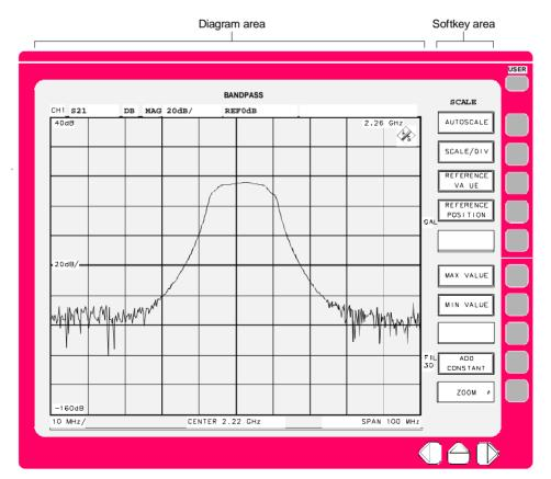
Fig. 2-12 General setup of the screen
