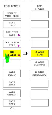
The *DEF X-AXIS* softkey opens the submenu for scaling the abscissa. Scaling parameters are
