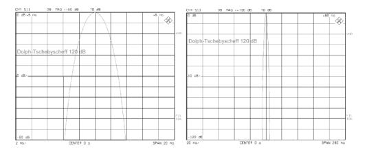
As for all other gates, the optimum solution depends on the specific measurement task. In general, a compromise must be found between either high time resolution or good signal suppression in the time domain, or between either low sidelobes or a narrow main lobe in the frequency domain.
