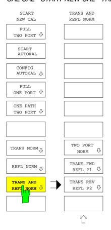
The TRANS AND REFL NORM softkey opens a menu for selecting a combined normalization calibration for transmission and reflection measurements.
