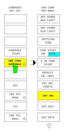
The *DEF COMP PNT MEAS* softkey opens the submenu for setting the parameters which define compression point measurements.
