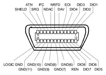
Fig. A-1 Pin assignment of IEC-Bus interface
