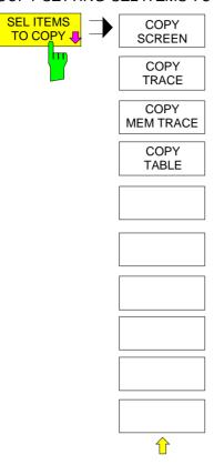
The SEL ITEMS TO COPY submenu comprises the four softkeys COPY SCREEN, COPY TRACE, COPY MEM TRACE and COPY TABLE. With these softkeys you can select the displayed elements to be printed.
