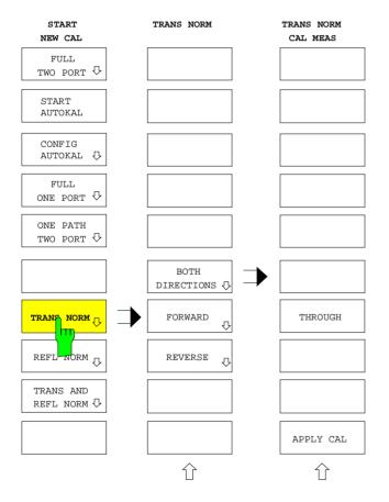
The TRANS NORM softkey calls the menu transmission normalization measurements. The measurement signal normalized in both (BOTH DIRECTIONS) or in one direction (FORWARD, REVERSE, see Section 2.15.1.1.7, "Unidirectional Two-port Calibration").
