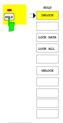
The functions of the *HOLD* menu disable either a subset of the control elements or the complete instrument control in order to prevent parameters from being changed by mistake.
