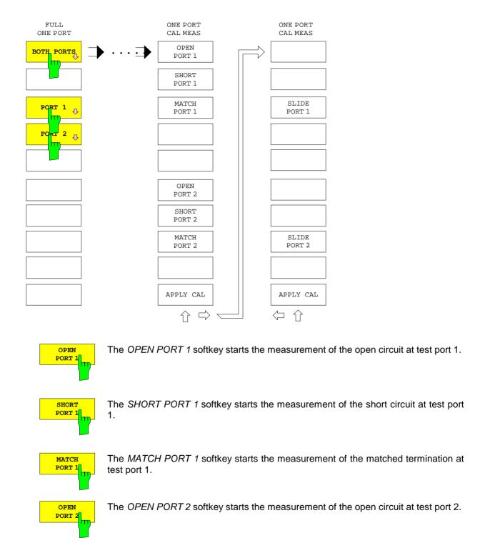
The SHORT PORT 2 softkey starts the measurement of the short circuit at test port
