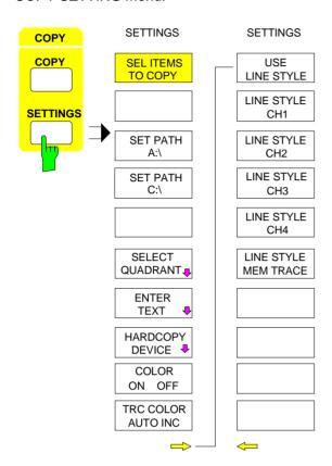
SETTINGS opens a configuration menu for the output of graphics, parameter lists and test reports to a printer, plotter or in the form of files.
