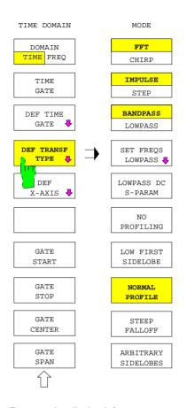
The *DEF TRANSF TYPE* softkey opens the submenu where the transformation type can be selected:
