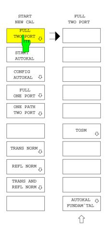
The *FULL TWO PORT* softkey selects the complete two-port calibration mode.
