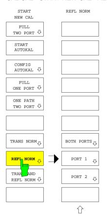
The REFL NORM softkey starts a reflection normalization calibration measurement.
