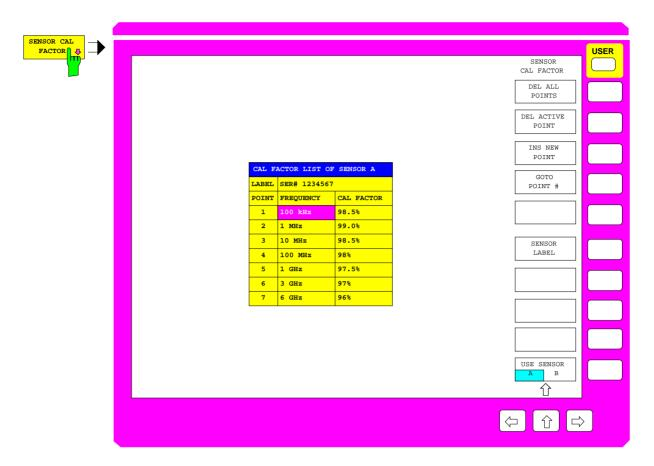
Fig. 2-42 Entry of a frequency-dependent calibration factor
