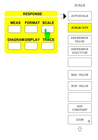
The *SCALE* key opens a menu scaling the test diagram in the active display channel.
