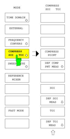
The COMPRESS SOI TOI softkey opens the menu providing operating modes used to determine quantities describing the nonlinear features of a DUT. These operating modes require the option "Nonlinear Measurements" (ZVR-B5).
