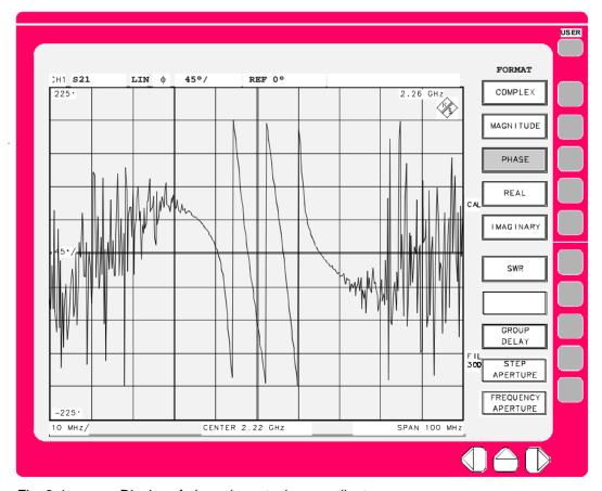
Fig. 2-4 Display of phase in cartesian coordinates
