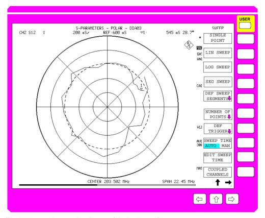
Fig. 2-17 Linear polar diagram (single channel)
