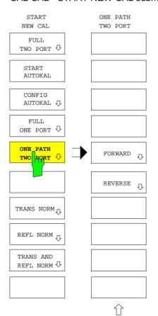
The ONE PATH TWO PORT softkey opens the menu for unidirectional two-port calibration.
