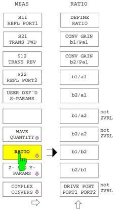
The *RATIO* softkey opens a submenu that selects ratios of the wave amplitudes received by the network analyzer as measured quantities.
