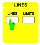
The *LINES* key group comprises the *LINES* and *LIMITS* keys. These keys provide auxiliary lines which make the evaluation of the trace easier.
