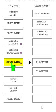
The MOVE LINE softkey opens a submenu which allows for moving limit lines.
