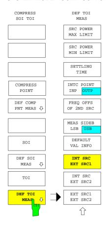
The *DEF SOI MEAS* softkey and *DEF TOI MEAS* open submenus for the setting of the parameters that define the second and third order intercept measurement.
