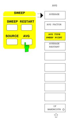
The AVG opens the menu containing all setting functions which refer to the measurement bandwidth.
