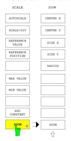
The ZOOM softkey opens a submenu where any segment of the test diagram in the active display channel can be magnified.
