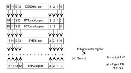
Fig. 3-3 The status register model
