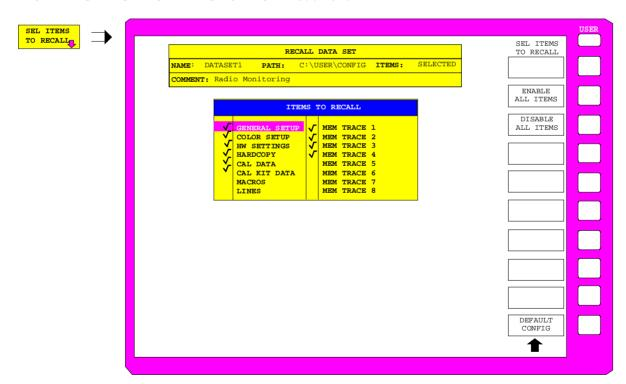
Fig. 2-32 Selecting partial data sets to be recalled
