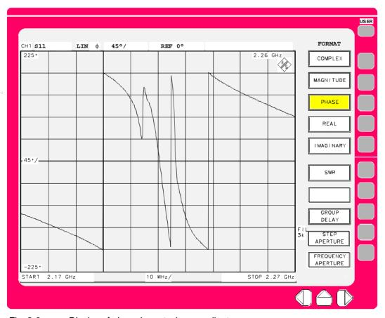
Fig. 2-6 Display of phase in cartesian coordinates
