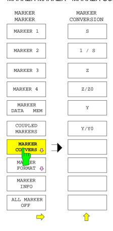
The MARKER CONVERS softkey opens a submenu in which the conversions of the marker values of the active display channel are set
