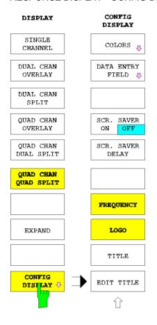
The CONFIG DISPLAY softkey calls a menu which sets the characteristics of the graphic elements of the display.
