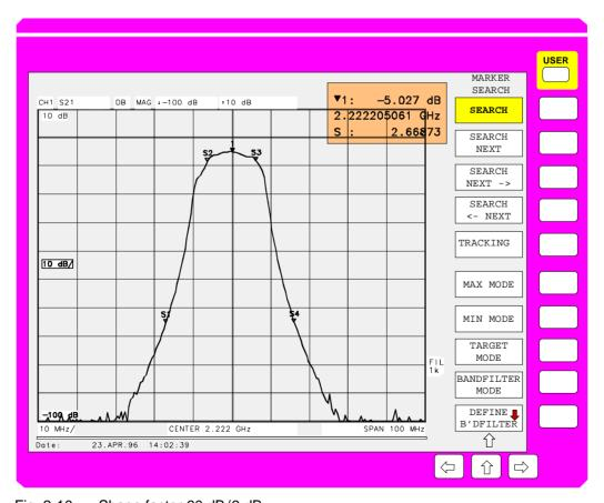
Fig. 2-10 Shape factor 60 dB/3 dB
