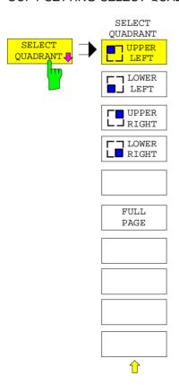
With the functions of the *SELECT QUADRANT* menu, the location of the displayed screen graphics on the printed page can be selected.
