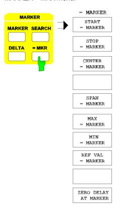
The = *MKR* key opens a menu where the stimulus or measured values of the last active marker or delta marker are assigned to specific parameters.
