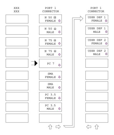
The type and order of the connectors shown in this menu are different for the different models of the ZVx family. The connector types used for the instrument test ports always come at the uppermost position.
