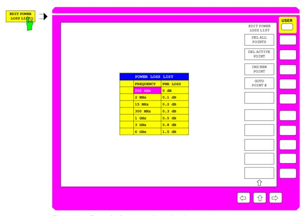
Fig. 2-43 Entry of a frequency-dependent loss
