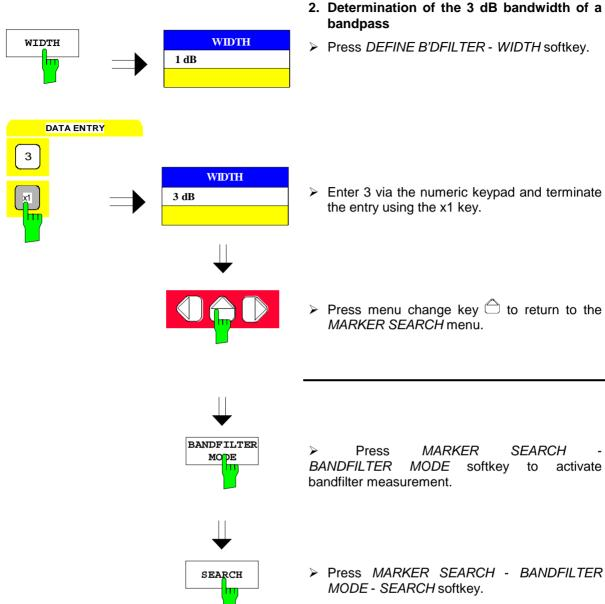
Two auxiliary markers are now displayed on the trace at the determined bandwidth points, one marker at the determined center frequency. The corresponding bandwidth is marker-info indicated in the line (see Fig. 2-8).
