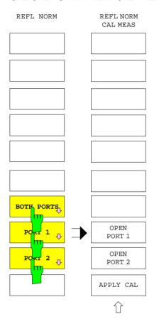
The PORT 1, PORT 2 and BOTH PORTS softkeys open the corresponding submenus for performing a reflection normalization at test port 1, test port 2 or at both test ports.
