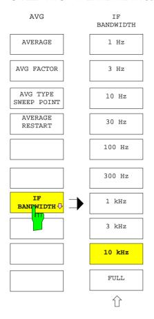
The *IF BANDWIDTH* softkey calls the submenu for setting the bandwidth of the digital receiver filter on the intermediate frequency.
