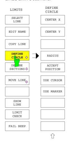
The *DEFINE CIRCLE* softkey calls a submenu for definition of a limit line in a circular diagram.
