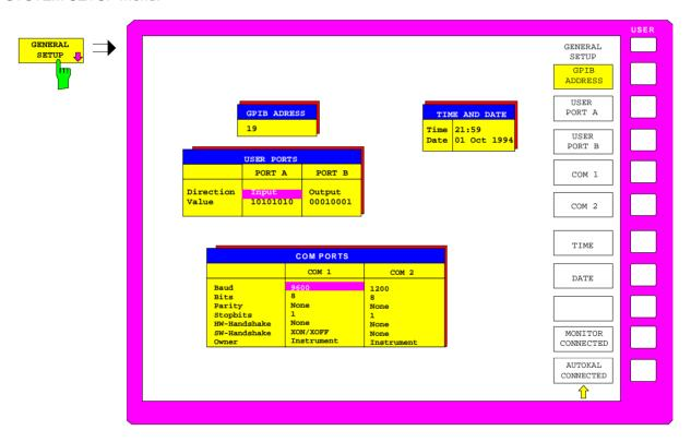
Fig. 2-23 Setting general parameters of the instrument
