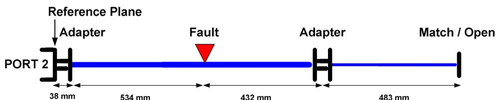
To prepare the distance-to-fault measurement, first perform a full one-port calibration at PORT 2:
