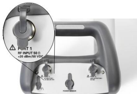
Connect a cable or DUT to the RF input with an N connector. Use a cable to connect the DUT to the R&S ZVH, if necessary.
