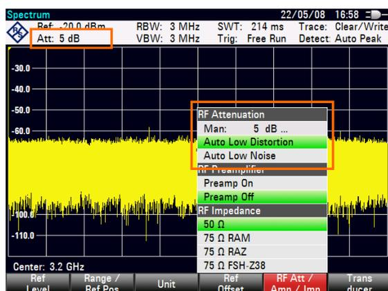
You can also set the attenuation manually. The R&S ZVH provides attenuation in the range from 0 to 40 dB in 5 dB steps.
