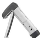
When laid out flat for operation from above, the R&S ZVH is still tilted slightly because of the grip on its top. This position provides the optimum viewing angle for the display.
