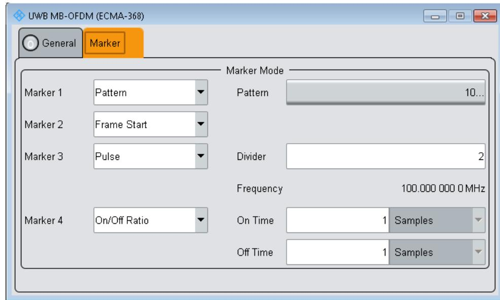
This tab provides access to the settings necessary to select and configure the marker output signal.
