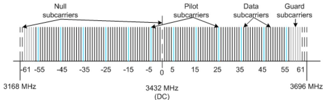
Figure 2-3: Structure of UWB MB-OFDM Signal
