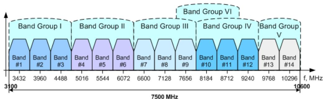
Figure 2-1: MB-OFDM Frequency Band Plan
