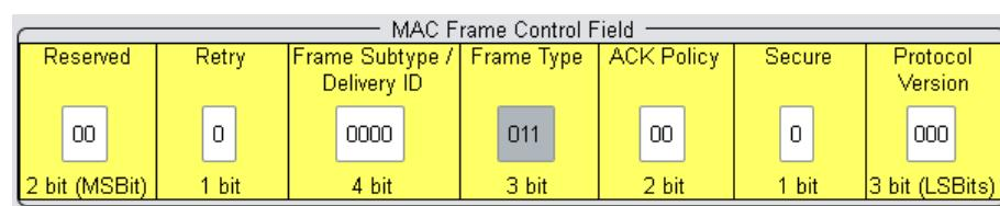
The value of parameter "Frame Control" is automatically set according to the settings for the "MAC Frame Control Field" and vice versa.
