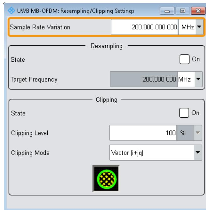
This tab provides access to the settings necessary to configure the sample rate variation, the resampling and clipping.
