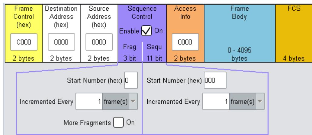
E.g. if it is to be simulated that some frames are received incorrectly or if the response of the receiver must be tested when the same frame arrives several times, the number of frames required to increment the sequence number can be set to 2.
