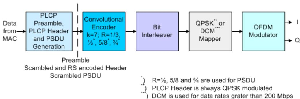
**Figure 2-8: Principle of UWB MB-OFDM signal generation**
