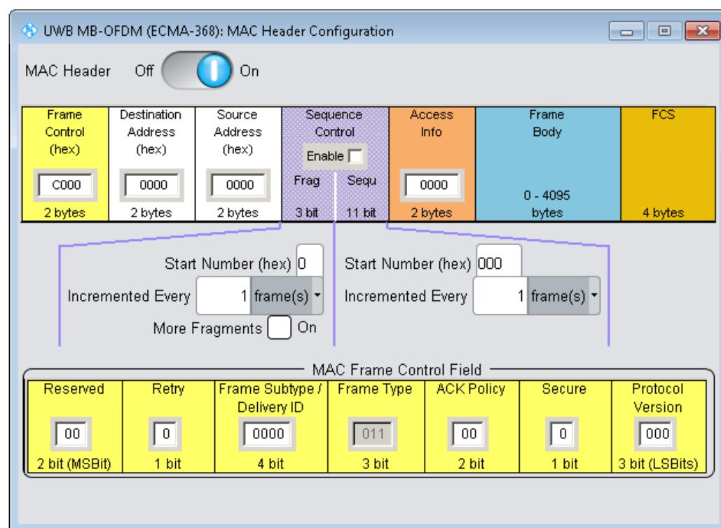
The dialog contains the settings necessary for MAC header configuration.
