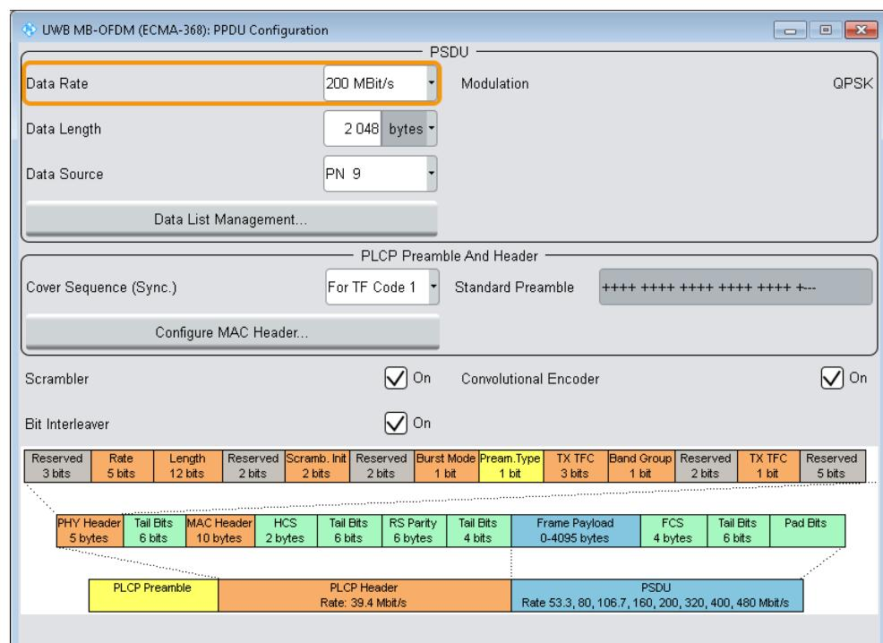
This dialog comprises the settings to select and configure the PSDU data part, the PLCP Preamble and PLCP Header. It enables you to activate the scrambler, bit interleaver and convolution encoder. The graph in the lower sections illustrates the structure of the PPDU.
