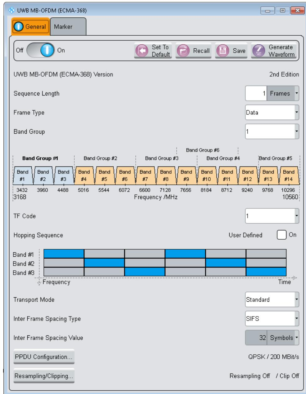
This dialog contains the standard general settings, the default and the "Save/Recall" settings. It enables you to select the sequence, frame and band group parameters, and provides access to dialogs with further settings.
