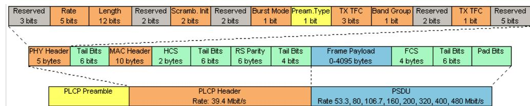
**Figure 2-7: UWB MB-OFDM Frame Structure**
