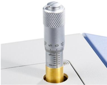
R&S SMZ instruments with mechanical level control are equipped with a power adjustment screw on top.
