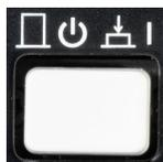
The switch turns on the internal modules of a frequency multiplier, or disconnects the instrument from the power supply.
