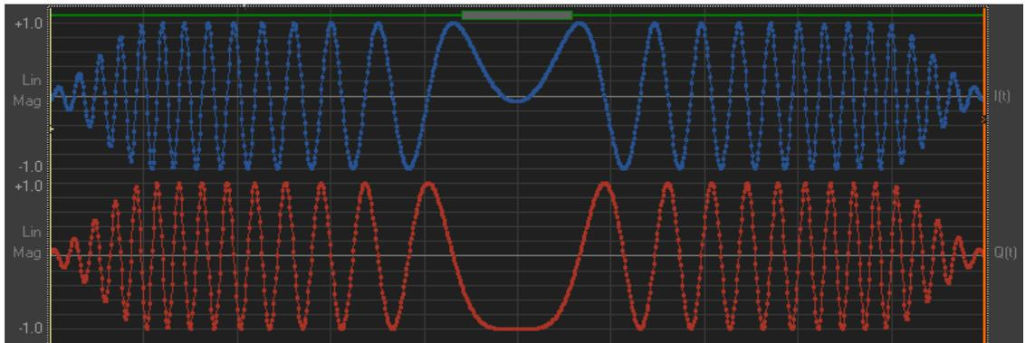
Fig. 38: I/Q waveform view of a chirped signal
