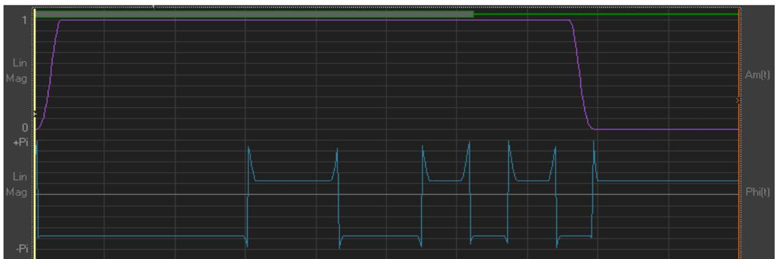
Fig. 39: Polar view of a BPSK modulated signal
