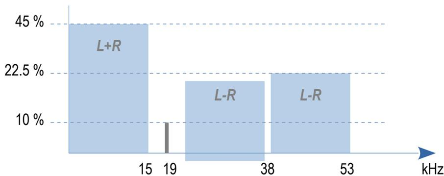
The stereophonic multiplex signal contains the sum of the left and right audio channel, a pilot tone of 19 kHz and a 38 kHz carrier that is analog modulated with the audio difference signal.
