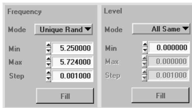
Fig. 54: Filling an RF List
