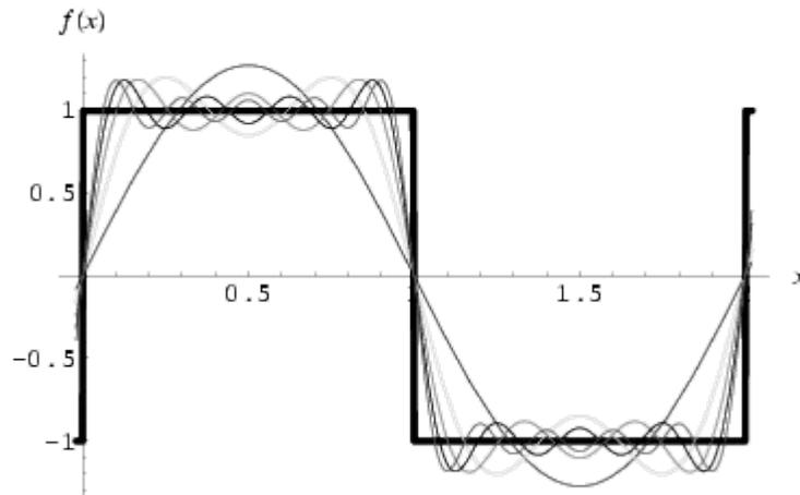
The figure shows a Fourier series of a square wave and can be described by the following equation:
