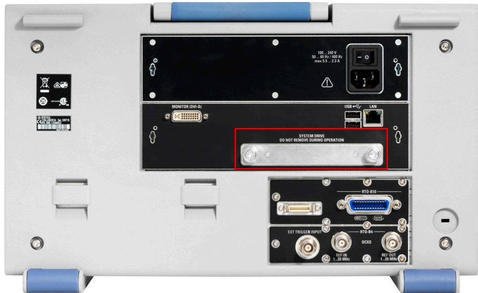
Figure 5-1: Location of the R&S RTO HDD/SSD
