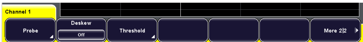
Fig. 5-2: Menu: "Probe" and "Threshold" open submenus, "More" switches the menu pages
