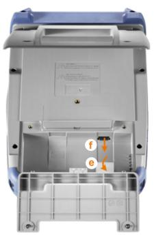
Figure 5-2: Removing of the micro SD card
