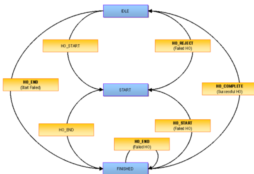
Figure 12-206: State machine illustrating handover procedure
