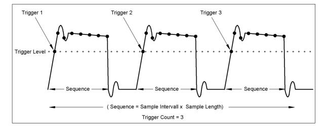
Fig. 4-6 Measurement repetition
