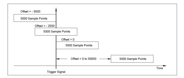
Fig. 4-5 Pre-trigger and post-trigger acquisition
