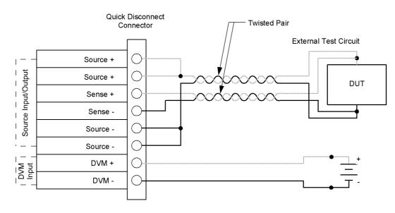
Fig. 4-2 Four-wire sense connection
