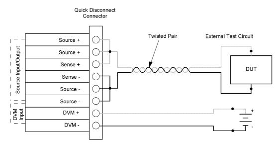
Fig. 4-3 Local sense connections
