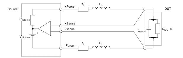
Fig. 3-4 Circuit diagram: Mobile phone connected to the NGMO2
