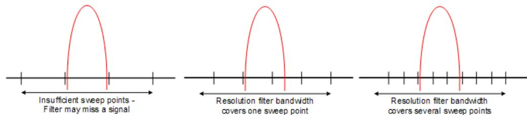
The resolution bandwidth should cover at least one sweep point (more is better). If this condition is not met, signals or interferences could be missed during final evaluation of narrowband interferers.
