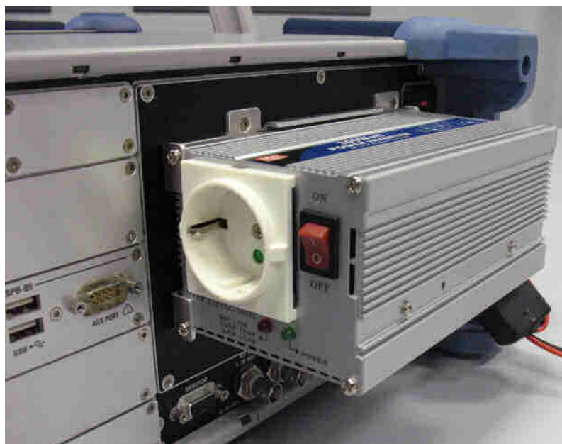
Figure 1-1: Installation of the DC power supply
