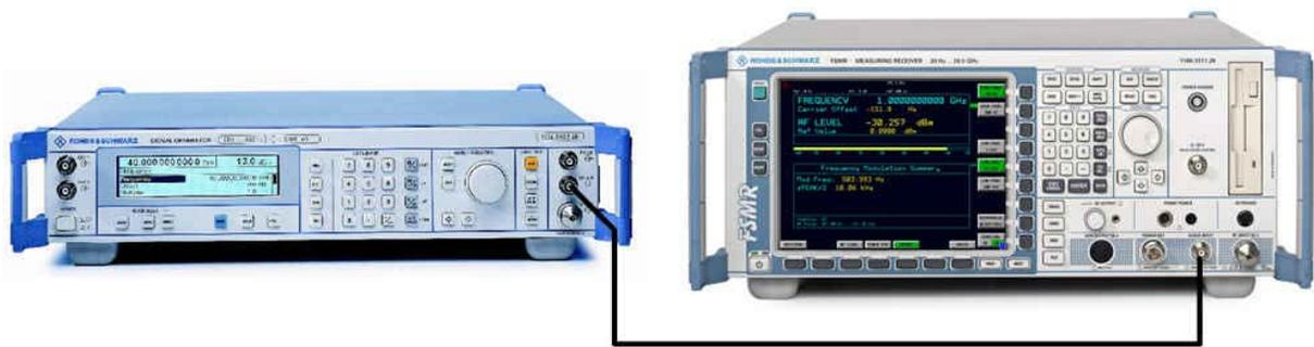
Fig.2-13 Audio measurement setup
