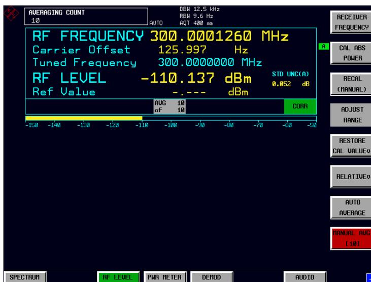
Fig.2-7 Tuned RF Level measurement at low levels
