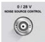
Output connector for an external noise source
