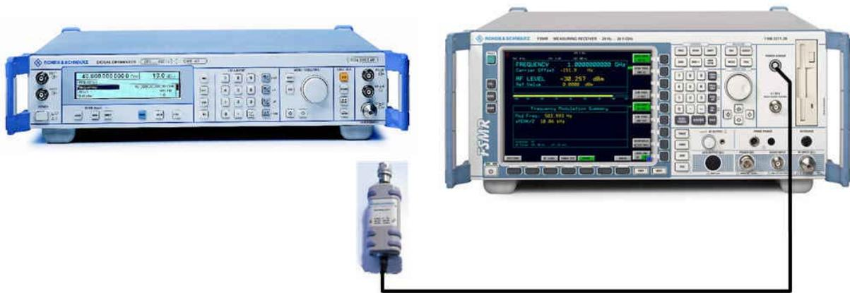
Fig.2-2 RF Power measurement setup
