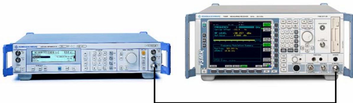
Fig.2-9 AM modulation measurement setup
