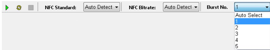
The size of the dropdown menu corresponds to the number of NFC bursts that the R&S FS-K112PC has detected in the I/Q data. For example, if the signal contains five bursts, the dropdown menu contains five entries.
