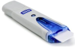
When you connect the reader to the computer, MS Windows automatically installs the necessary drivers. If not, you can install the drivers manually from the software CD. The required files are stored in the directory `\Install\USB SmartCard Reader Driver Files`. The driver files are named according to the processor architecture for which they are designed. (OMNIKEY3x21\_x86 or OMNIKEY3x21\_x64).
