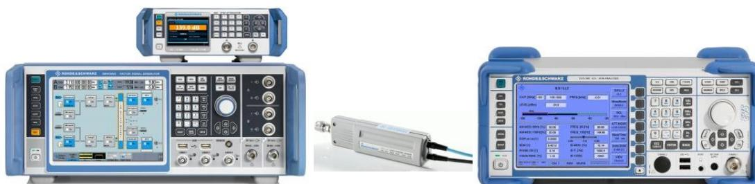
The Vector Signal Generator SMW200A generates arbitrary signals with very high linearity and very low distortion. Avionic signals are calculated on the PC and can be generated with the required accuracy. While the predecessor of the EVS-Z11 needed a reference receiver (FMAV) to fine adjust the avionic signals, the SMW can go without.
