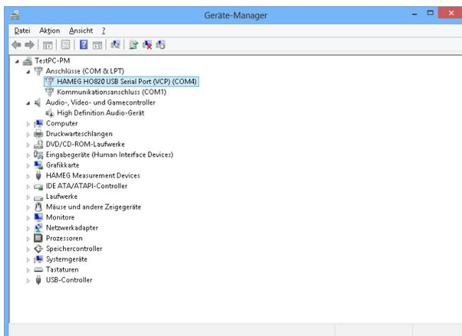
Fig. 4.5: VCP installed
