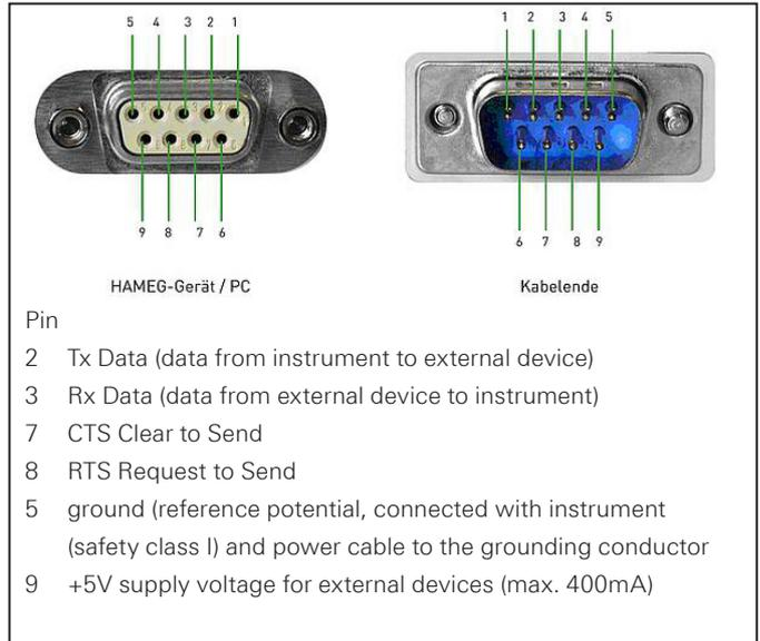
Fig. 1.2: Pin assignment of the RS-232 interface
