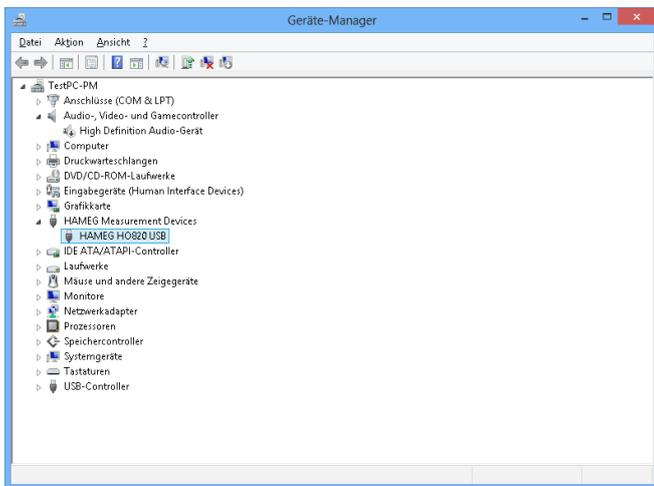
Fig. 3.11: Instrument display in the device manager
