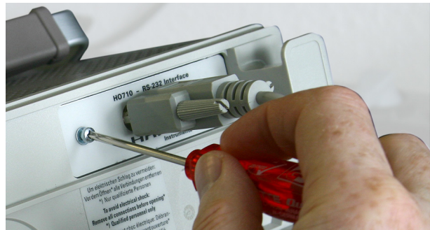
Fig. 2.1: Remove fastening screws
