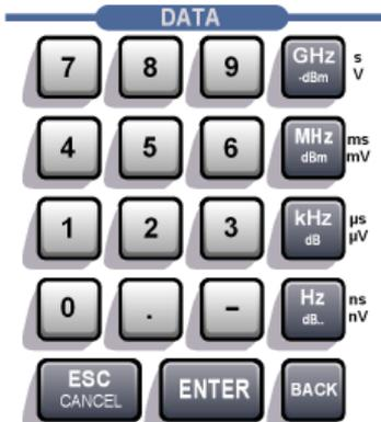
The keypad is used to enter numeric parameters. It contains the following keys:
