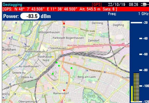
With this Application Sheet we give a step by step introduction how to setup and perform an outdoor coverage measurement using the R&S FSH Handheld Spectrum Analyzer together with the HA-Z240 GPS receiver.
