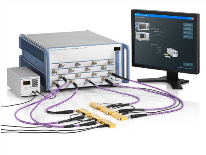
Multiport device test setup – scenario 1 (based on R&S®ZNB true multiport network analyzer).
