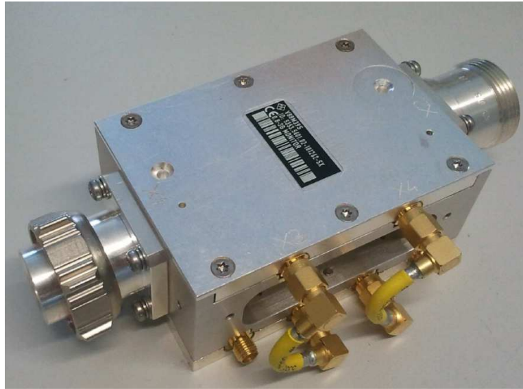
Fig. 15: Coupling attenuation -58 dB @ 1 GHz, directivity < -26 dB.
