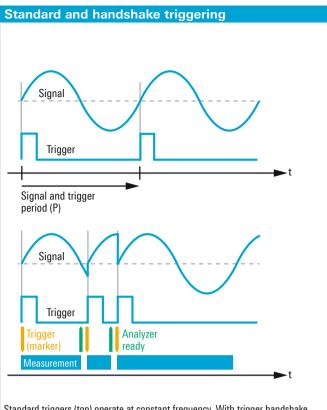
Standard triggers (top) operate at constant frequency. With trigger handshake (bottom) the generator restarts the waveform to initiate the trigger event when the analyzer is ready for the next measurement.
