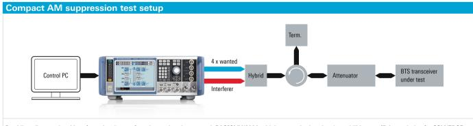
Providing all wanted and interferer signals out of one box makes the two-path R&S<sup>®</sup>SMW200A with its extensive baseband capabilities an efficient solution for GSM/EDGE AM suppression conformance tests.
