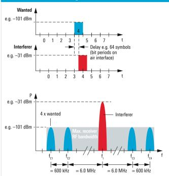
Several properly synchronized vector signal generators (VSGs) provide the required wanted signals to the receiver under test at a certain power level and frequency. An additional VSG delivers the specified modulated interfering signal (at a significantly higher power level) to the receiver.
