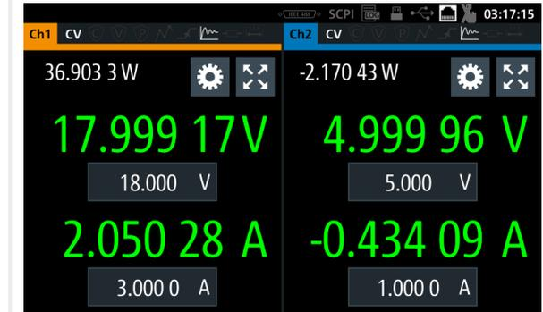
The linear design of the output stages reduces residual ripple and noise to a minimum and makes them perfect for the development of power amplifiers and MMICs.
