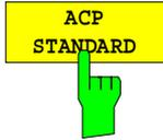
*ACP STANDARD* soft key activates the selection of a digital mobile-radio standard. The parameters for the adjacent channel power measurement are set according to the regulations of the selected standard.
