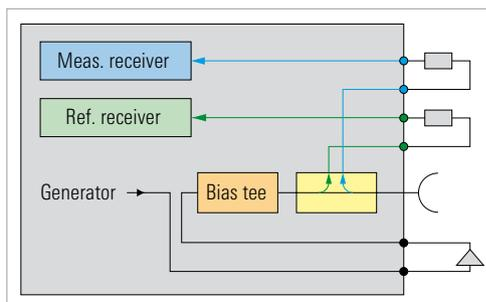
*Internal combiner and generator step attenuators for the R&S®ZVT20*
