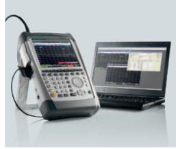
The R&S®ZVHView software with the wizard and report generator tool is included as standard. It is primarily used to centrally prepare measurements and postprocess results.
