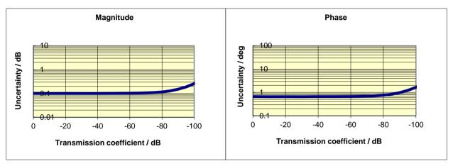
Typical accuracy of transmission magnitude and transmission phase measurements of the R&S<sup>®</sup>ZVA40 in the frequency range 700 MHz to 24 GHz
