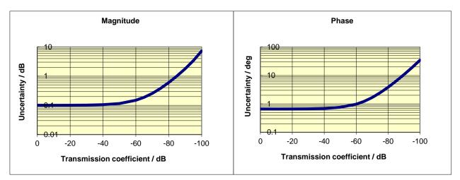
Typical accuracy of transmission magnitude and transmission phase measurements of the R&S<sup>®</sup>ZVA24 in the frequency range 10 MHz to 700 MHz
