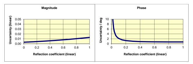
Typical accuracy of reflection magnitude and reflection phase measurements of the R&S<sup>®</sup>ZVA8 in the frequency range 1 MHz to 8 GHz, of the R&S<sup>®</sup>ZVA24 in the frequency range 50 MHz to 24 GHz, of the R&S<sup>®</sup>ZVA40 in the frequency range 50 MHz to 40 GHz, of the R&S<sup>®</sup>ZVA50 in the frequency range 50 MHz to 50 GHz and of the R&S<sup>®</sup>ZVA67 in the frequency range 50 MHz to 67 GHz
