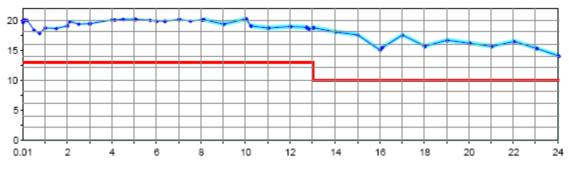
Maximum output power in dBm versus frequency in GHz of the R&S®ZVA24
