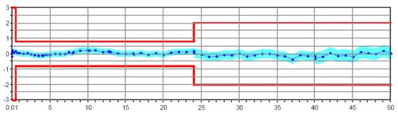
Output power accuracy in dB versus frequency in GHz of the R&S®ZVA50
