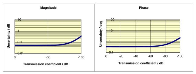
Typical accuracy of transmission magnitude and transmission phase measurements of the R&S<sup>®</sup>ZVA8 in the frequency range 50 MHz to 8 GHz
