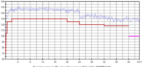
Dynamic range in dB versus frequency in GHz of the R&S<sup>®</sup>ZVA40
