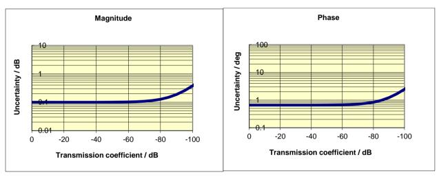
Typical accuracy of transmission magnitude and transmission phase measurements of the R&S<sup>®</sup>ZVA24 in the frequency range 700 MHz to 24 GHz
