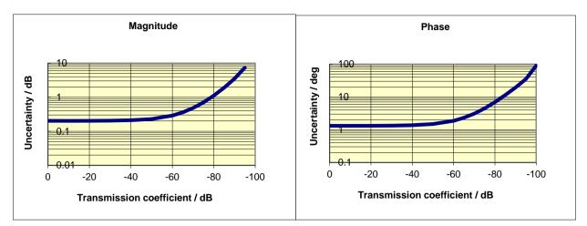
Typical accuracy of transmission magnitude and transmission phase measurements of the R&S<sup>®</sup>ZVA50 and R&S<sup>®</sup>ZVA67 in the frequency range 10 MHz to 700 MHz
