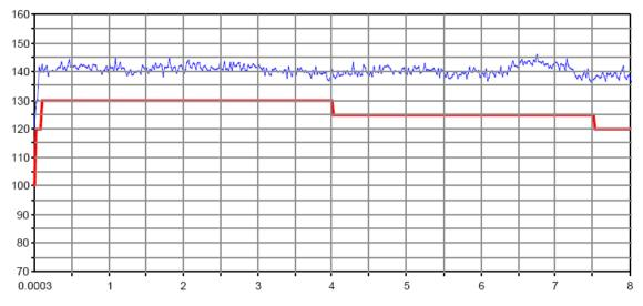
Dynamic range in dB versus frequency in GHz of the R&S<sup>®</sup>ZVA8
