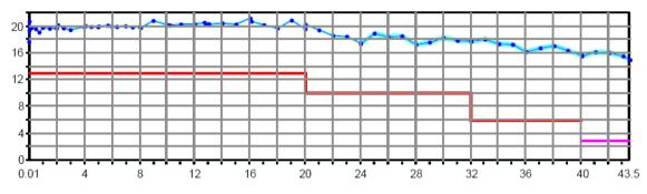
Maximum output power in dBm versus frequency in GHz of the R&S<sup>®</sup>ZVA40
