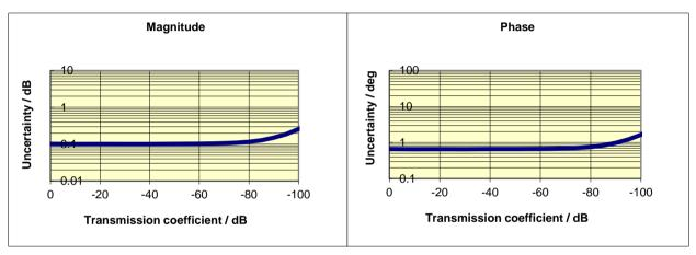
Typical accuracy of transmission magnitude and transmission phase measurements of the R&S<sup>®</sup>ZVA50 and R&S<sup>®</sup>ZVA67 in the frequency range 700 MHz to 24 GHz
