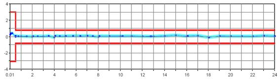
Output power accuracy in dB versus frequency in GHz of the R&S<sup>®</sup>ZVA24
