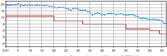
Maximum output power in dBm versus frequency in GHz of the R&S®ZVA67
