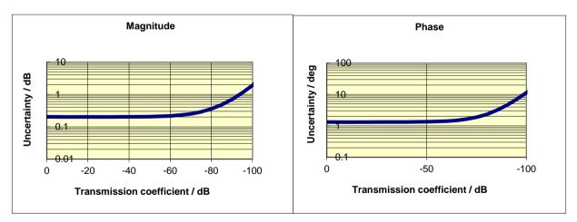
Typical accuracy of transmission magnitude and transmission phase measurements of the R&S<sup>®</sup>ZVA50 and R&S<sup>®</sup>ZVA67 in the frequency range 24 GHz to 50 GHz
