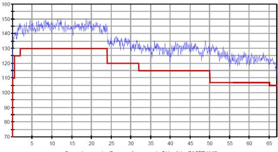
Dynamic range in dB versus frequency in GHz of the R&S<sup>®</sup>ZVA67
