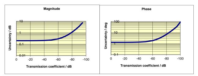
Typical accuracy of transmission magnitude and transmission phase measurements of the R&S<sup>®</sup>ZVA40 in the frequency range 10 MHz to 700 MHz
