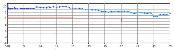
Maximum output power in dBm versus frequency in GHz of the R&S<sup>®</sup>ZVA50
