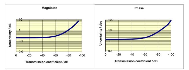
Typical accuracy of transmission magnitude and transmission phase measurements of the R&S<sup>®</sup>ZVA67 in the frequency range 50 GHz to 67 GHz
