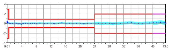
Output power accuracy in dB versus frequency in GHz of the R&S®ZVA40
