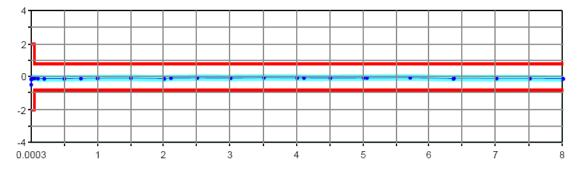
Output power accuracy in dB versus frequency in GHz of the R&S<sup>®</sup>ZVA8
