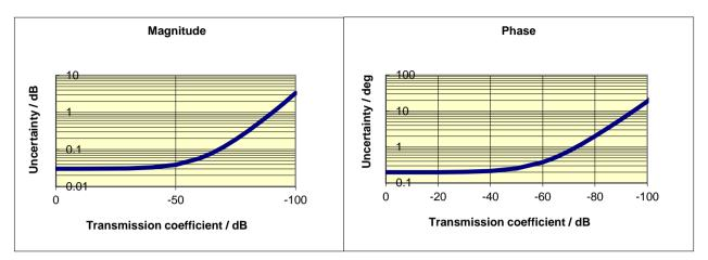
Typical accuracy of transmission magnitude and transmission phase measurements of the R&S<sup>®</sup>ZVA8 in the frequency range 300 kHz to 50 MHz
