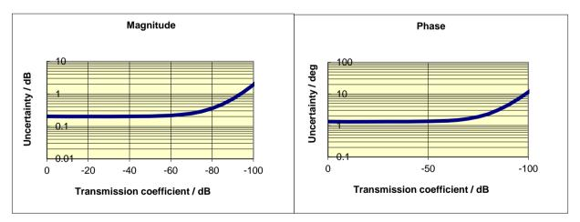
Typical accuracy of transmission magnitude and transmission phase measurements of the R&S<sup>®</sup>ZVA40 in the frequency range 24 GHz to 40 GHz
