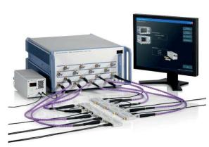
Control up to 48 calibration modules with one single controller; use multiple controllers for higher port count. Ensure stable, repeatable accuracy by easy and fast recalibration
