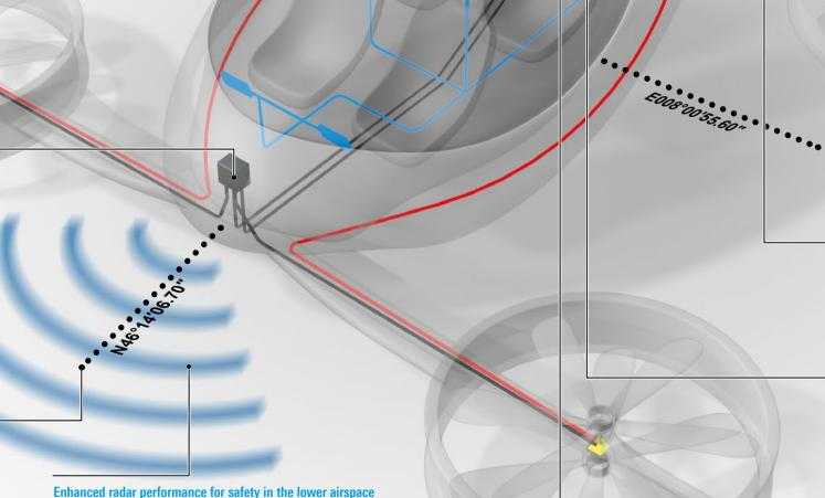
Radar is the first choice for onboard sensors, enabling detection and
