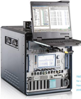
R&S®UCS-Compact radio test set for on-site maintenance and overhaul (drawer monitor in operation position).
