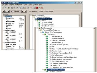
Predefined test sequences make it easy to switch between different test levels.
