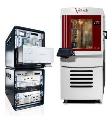
The test equipment used for I-level servicing of R&S®M3AR radios consists of the R&S®UCS-Base radio test set and the radio's harness and connectors. The R&S®UCS-Base has been designed based on the R&S®UCS test system family, the platform used in Rohde & Schwarz production and repair facilities. It ensures high performance during testing and availability of up-to-date test software.
