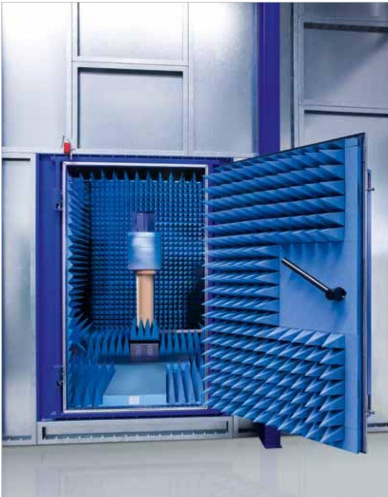
Anechoic test chamber for MIMO OTA measurements.
