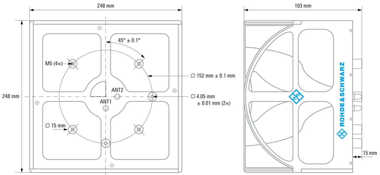
Mounting interface of the R&S®TC-TA18 cross-polarized Vivaldi test antenna.
