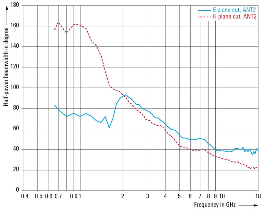
Half-power beamwidth of the R&S<sup>®</sup>TC-TA18 cross-polarized Vivaldi test antenna; port ANT2 (meas.).
