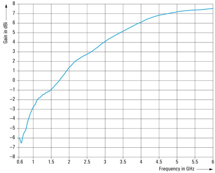
Gain of the R&S<sup>®</sup>TC-CA6 linear-polarized communications antenna (meas.).
