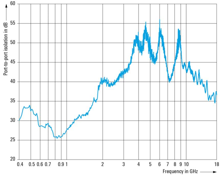
Port-to-port isolation of the R&S<sup>®</sup>TC-TA18 cross-polarized Vivaldi test antenna (meas.).
