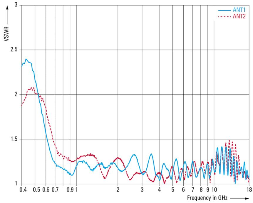
VSWR of the R&S<sup>®</sup>TC-TA18 cross-polarized Vivaldi test antenna (meas.).
