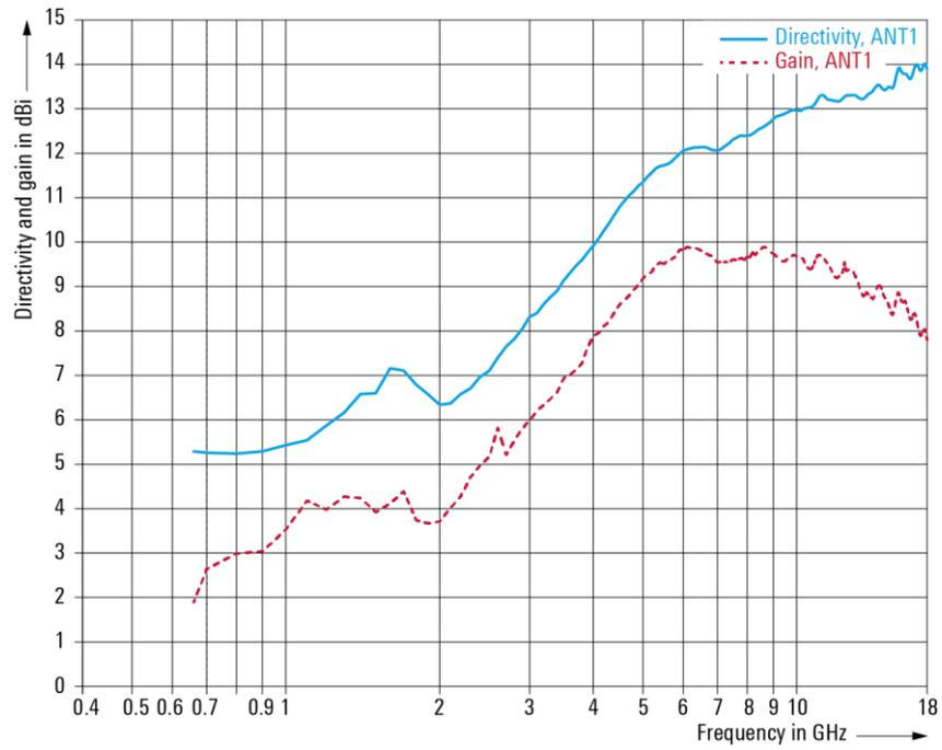
Directivity and gain of the R&S®TC-TA18 cross-polarized Vivaldi test antenna; port ANT1 (meas.).
