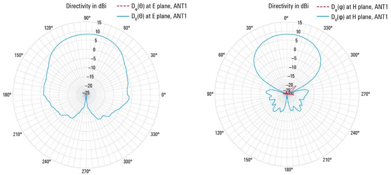
Partial directivity of the R&S<sup>®</sup>TC-TA18 cross-polarized Vivaldi test antenna at 3 GHz; port ANT1 (meas.).
