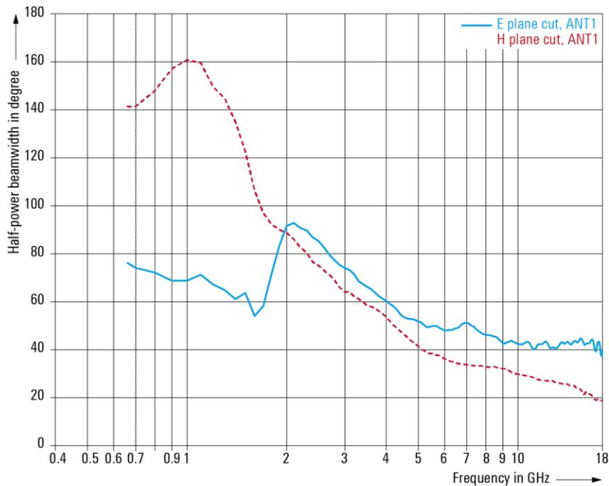
Half-power beamwidth of the R&S®TC-TA18 cross-polarized Vivaldi test antenna; port ANT1 (meas.).
