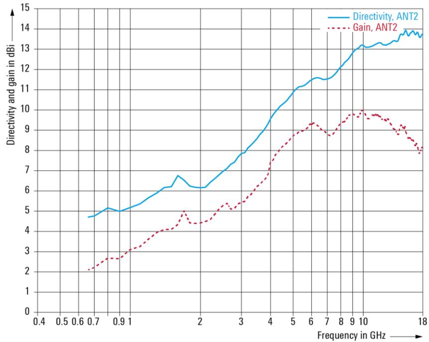
Directivity and gain of the R&S®TC-TA18 cross-polarized Vivaldi test antenna; port ANT2 (meas.).
