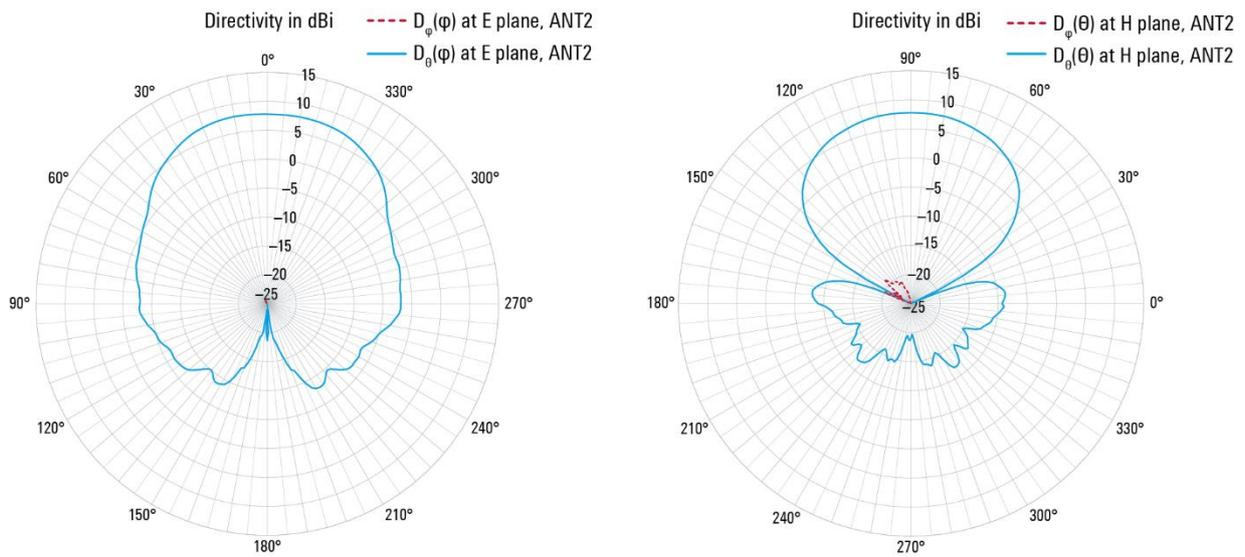
Partial directivity of the R&S<sup>®</sup>TC-TA18 cross-polarized Vivaldi test antenna at 3 GHz; port ANT2 (meas.).
