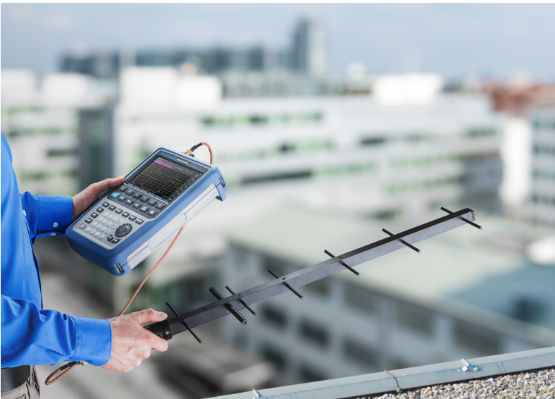
R&S®Spectrum Rider FPH 配备 R&S®HA-Z900 八木天线
