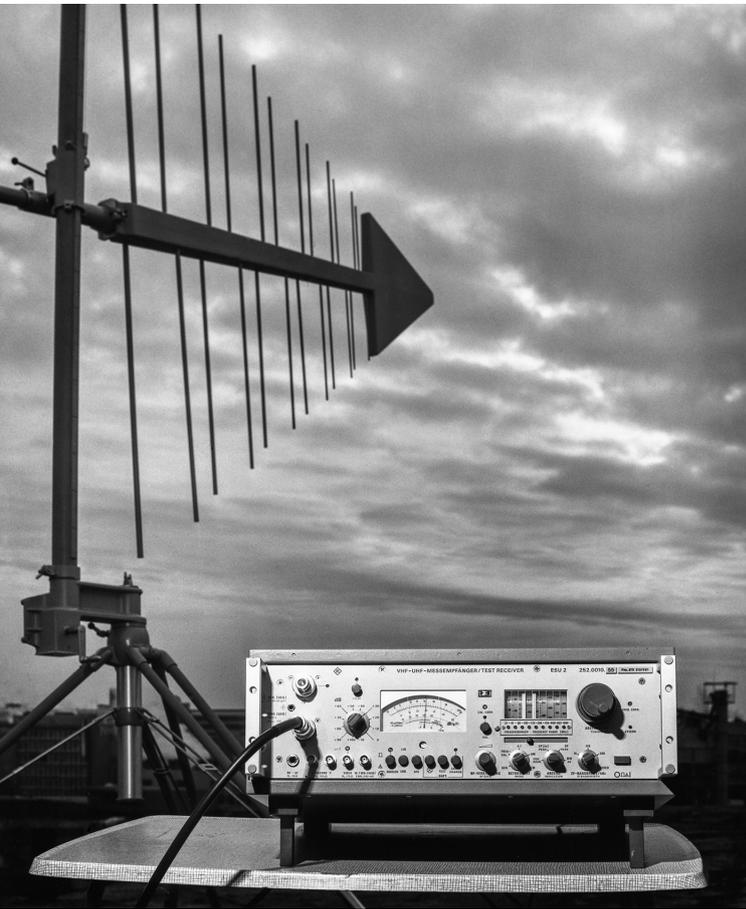
Fig. 7: HFU2 VHF/UHF field strength meter with ESU2 test receiver and HL023 log-periodic broadband antenna for 80 MHz to 1300 MHz.
