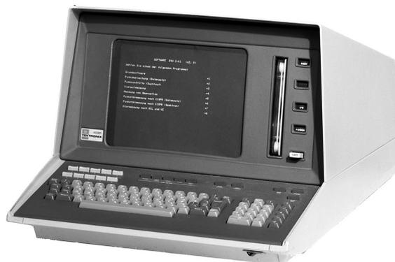
Fig. 8: MSUP VHF/UHF tester. The common instrument case contained the ESU2-Z4 IEC/IEEE bus adapter with built-in frequency counter, the EZP panorama adapter, the EZK frequency controller and the ESU2 measuring receiver (from top to bottom). The Tektronix 4051 desktop computer combined all this into an automated test setup.
