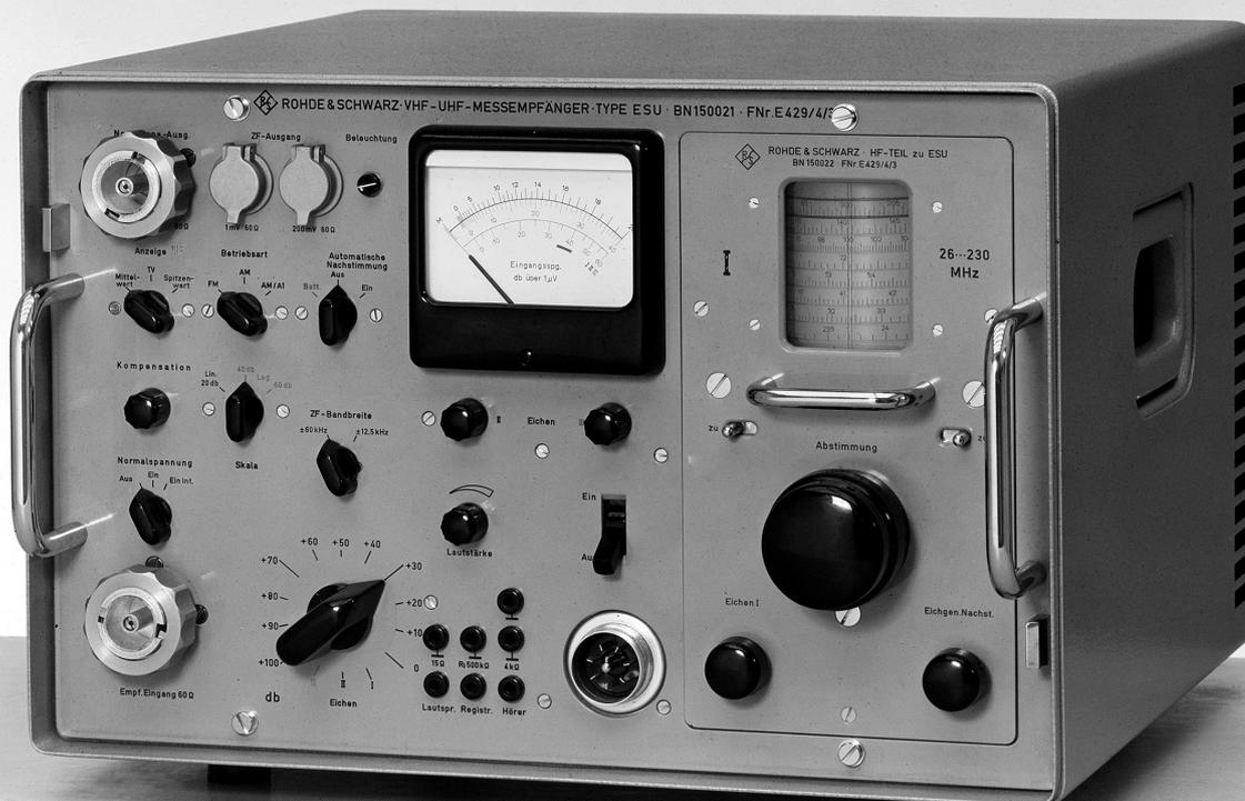
measuring frequency, was a major advancement. Operation was also simplified by selectable display ranges (linear 20 dB, logarithmic 40 dB or 60 dB), switchable average or peak value display, selectable passband (25 kHz or 120 kHz) and optional automatic frequency control.
