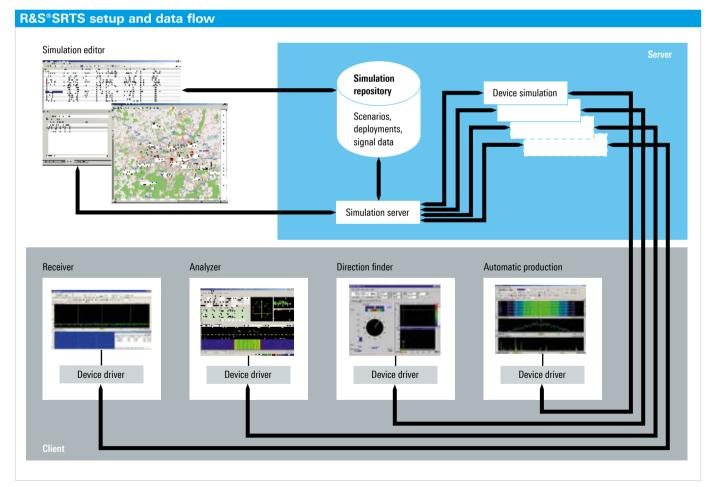
All signal scenario data (activity lists, spatial distribution and transmit parameters of the virtual transmitters as well as contents such as audio) is kept in a central storage. The central simulation server administers and distributes the virtual scenario created with the simulation editor and the scenario's contents to the connected device simulations. The graphical user interfaces (GUI) of the individual workstations set up the connection to the virtual devices via a LAN or WAN.
