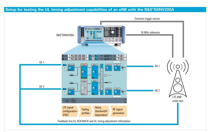
A two-path concept and the R&S°SMW-K55 and R&S°SMW-K69 software options make the R&S°SMW200A ideal for performing standard-compliant UL tests of eNBs in line with 3GPP TS 36.141, section 8.2.2 — using just one T&M instrument.
