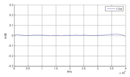
Measured frequency response of I/Q outputs.
