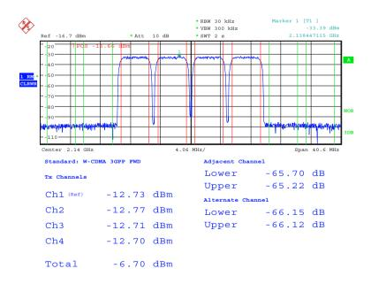
Measured ACPR for a 3GPP four-carrier signal with test model 1, 64 DPCH on each carrier (baseband gain: +3 dB).
