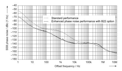
Measured SSB phase noise, f = 1 GHz, comparison of standard performance and performance with R&S<sup>®</sup>SMU-B22 option.
