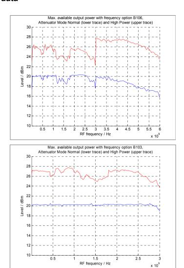
Measured maximum available output level versus frequency.
