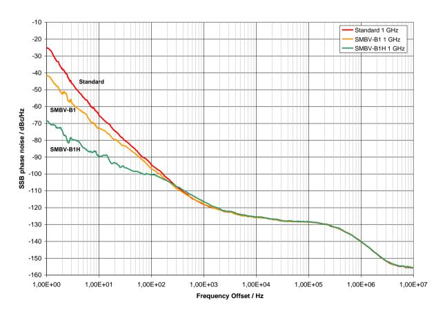
SSB phase noise comparison with standard internal reference, R&S®SMBV-B1, R&S®SMBV-B1H (meas.)
