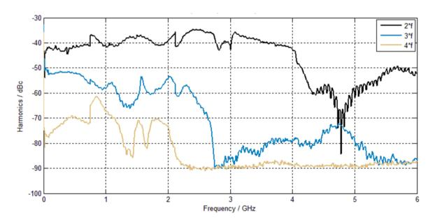
Harmonics versus carrier frequency at +18 dBm output level (meas.)
