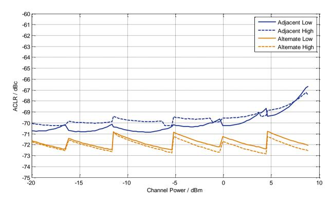
Digital standard 3GPP FDD test model 1, 64 DPCHs, ACLR as a function of carrier level at 2 GHz (meas.)
