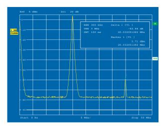
Spurious suppression of the internal baseband generators
