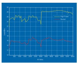
Typical maximum output power over frequency (with high-power output option)
