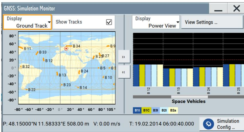
Combined B11, B1C, B2I, B2a and B3I simulation performed by the R&S®SMBV100B
