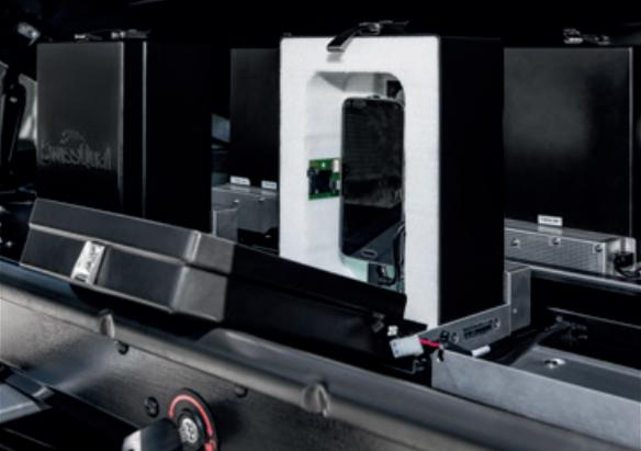
Thermal containment modules ensure uniform and stable conditions for benchmarking campaigns
