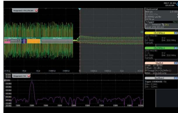
You can combine protocol decoding with other analysis tools. This spurious communications breakdown shows good data until it stops. The reason for the breakdown is a 2 MHz signal as seen in the FFT at the bottom part of the screen.
