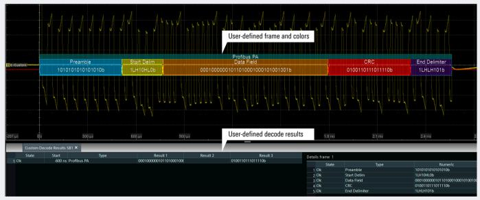
Custom trigger and decode for profibus PA
