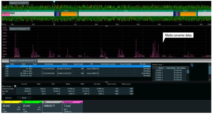
Example of bus timing measurements on a 100BASE-T1 bus
